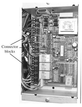
Fig. 11 Control module, showing connector blocks.
