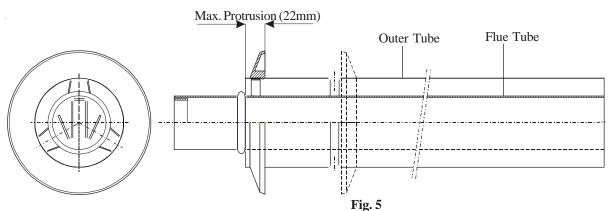
Horizontal Flue Terminal (Showing Maximum Protrusion)
